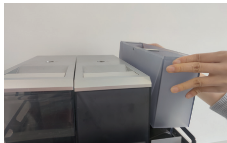
6. Attach the powder hopper
