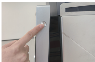
2. Press the screen power button
