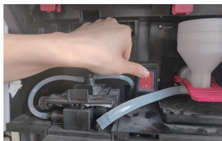
1. Lift the front operation panel and press the power switch
