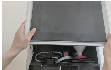
2. Lift the front operation panel
