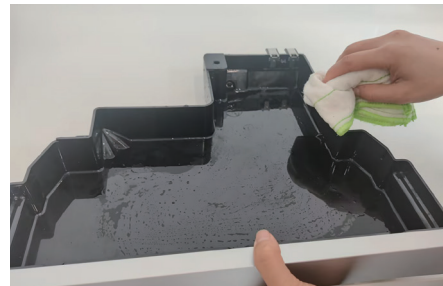
4. Dry and place the drip tray back
