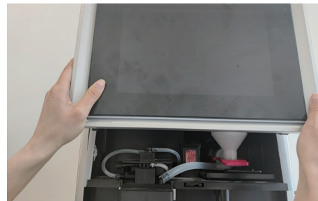
2. Lift the front operation panel
