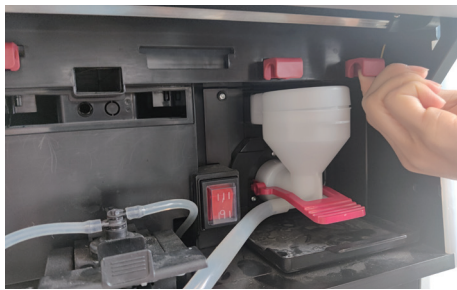
3. Pull the locking slide towards the forward if possible
