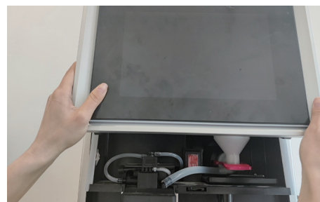
2. Lift the front operation panel
