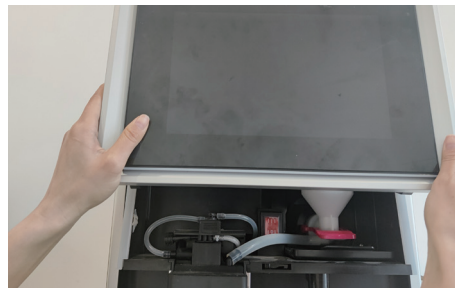
2. Lift the front operation panel
