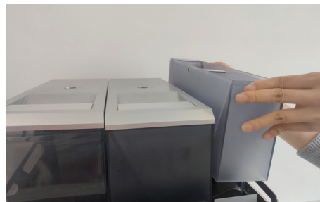
6. Attach the powder hopper
