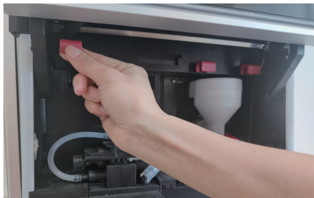
7. Push the locking slide all the way in
