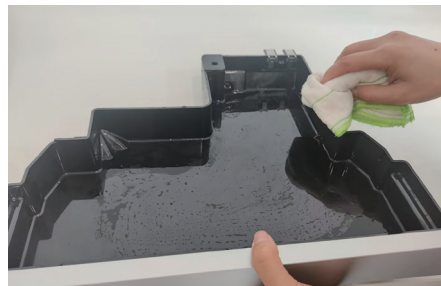
4. Dry and place the drip tray back
