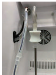
3. Connect milk hose (inlet) to metal milk hose
